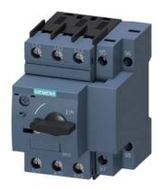
Circuit breaker size S00 for motor protection, CLASS 10 with overload relay function A-release 4.5...6.3 A N-release 82 A screw terminal Standard switching capacity
