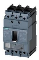
circuit breaker 3VA5 UL frame 125 breaking capacity class H 65kA @ 480 V 3-pole, line protection TM230, FTAM, In=35A overload protection Ir=35A fixed short-circuit protection Ii=5...10 x In nut keeper kit on both sides
