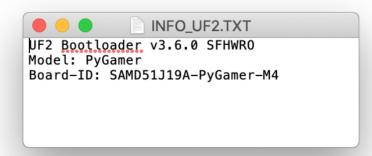
If the bootloader version you see is older than *v3.9.0*, you need to update. For instance, the bootloader above needs to be upgraded.
