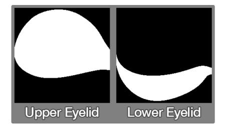
The white area — which should span the **entire 240 pixel width** — represents the extent of vertical motion, the "open-most" and "closed-most" range. The eyes won't hold the open-most position all the time when idle...the upper eyelid "tracks" the moving pupil, because that's how eyes work.
