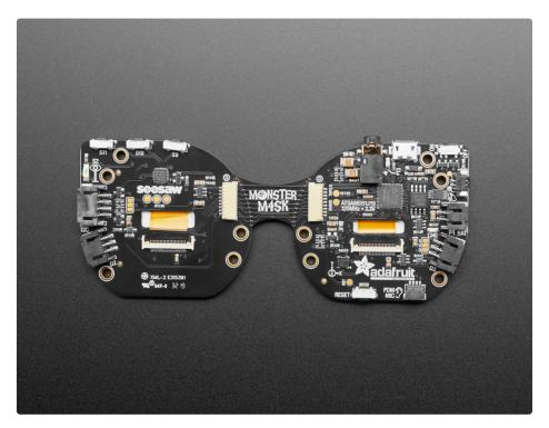
This unique design has the eyes at the same pupil-distance as a human (~63mm) but is designed so that the nose section can be broken apart with pliers/cutters and then wired together with a 9-pin JST SH cable up to 100mm long (https://adafru.it/FAZ) so the eyes can be re-positioned or freely attached.
