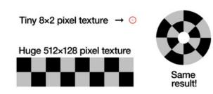
Eye textures can be any size (RAM permitting), on either axis...even down to a single pixel. When wrapping small images around the whole eye, **nearest-neighbor** sampling (no interpolation) is used. This can be exploited to create stylized blocky or grid designs...no need to waste space on a big image when just a few pixels will do.
