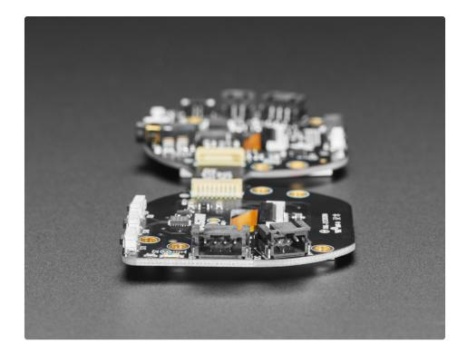
On each side are JST-PH plugs for connecting external devices. The 3-pin JSTs connect to analog/timer pins on the SAMD51, so you can use them for sensors or GPIO devices. The 4-pin JST connector connects to the I2C port and you can fit Grove connectors in it for additional hardware support. For the PDM mic port, you can use this cable (https://adafru.it/FA-) to wire to a PDM mic (https://adafru.it/FB0).
