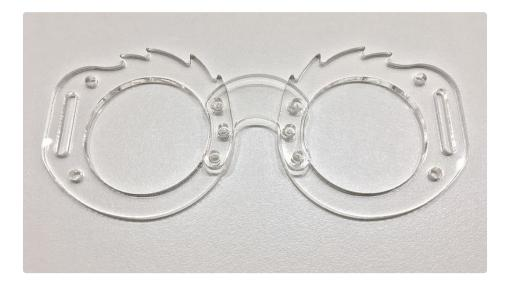
There is an optional extra **nose bridge** piece. If you have **split** your MONSTER M4SK apart and want to use it in its original shape again, this piece holds the frames at their original spacing. An optional **9-pin JST cable** must link the two boards, you'll need some **different length** M3 screws, and you **will not get the boopable nose** feature back.
