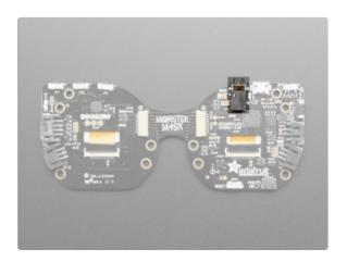
There is a **stereo headphone jack** on the top of the right side. This is connected to the two analog DAC pins on the SAMD51 - **AO** and **A1**
