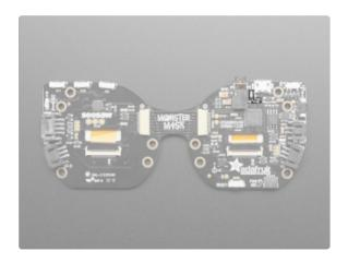
On the top of the right side, next to the USB connector, is a **little red LED** tied to pin **D13**. You can control it in your code. It pulses when the board is in bootloader mode.
