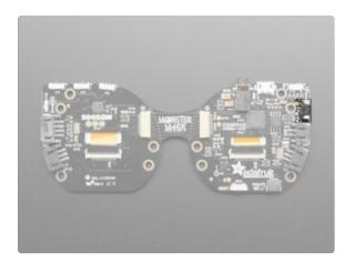
There is a mono speaker driver for smaller 8 ohm 1W speakers. Add a speaker using the Molex PicoBlade (https://adafru.it/C8p) speaker connector located on the right side of the board towards the top. The speaker is connected to the AO analog DAC, and can be enabled/disabled using the SPEAKER ENABLE pin (pin 20)
