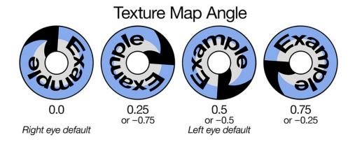
irisAngle and scleraAngle are a rotation offset in the clockwise direction, using either normalized floating point where 0.0=seam at top, 0.25=seam at right, 0.5=bottom, 0.75=left, and 1.0=back to top. You can also use integer units from 0 to 1024 (0=top, 256=right and so forth). Negative values are accepted for both the floating-point and integer modes, in which case the angle will be counter-clockwise.
