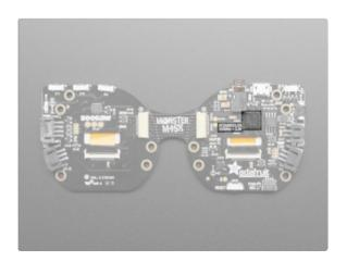
The main processor chip is the **ATSAMD51G19** Cortex M4 microcontroller running at 120MHz with 512KB Flash, and 192KB RAM.
