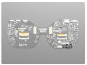
At the bottom on the right side is a **4 pin JST SH port** for connecting an optional **PDM microphone**. Note that the PDM microphone is connected to two SERCOM pins, and we use **SPI2** to read PDM data (if you think about it, PDM is just fixed-frequency SPI!) You *could* in theory turn this into an I2C or UART port. The SAMD51G19 chip used on this board does not support I2S, so we can't use I2S to read the PDM data.
