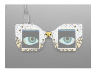
Front and center, is a **capacitive touch pad nose** this is connected to **D2**. It's not a *great* capacitive touch input, because of the zener diode on D2's protection circuitry, but it can detect presses with some startup-calibration. Use as an input.
