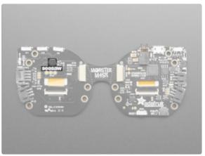
Towards the top center of the left side is the **seesaw chip**. This chip handles the tactile buttons and the light sensor. You can read the data from them using the I2C seesaw library and the pins specified. This is what lets us have only 9 wires to bridge the two halves of the PCB
