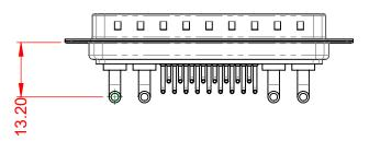
POWER/CO-AX CONTACT RATING:20A (CURRENT)(IF PRESENT)SIGNAL CONTACT CURRENT RATING:5A PER CONTACTSIGNAL CONTACT RESISTANCE:10mΩ MAX.INSULATOR RESISTANCE:5000MΩ min.DIELECTRIC5000MΩ min.
