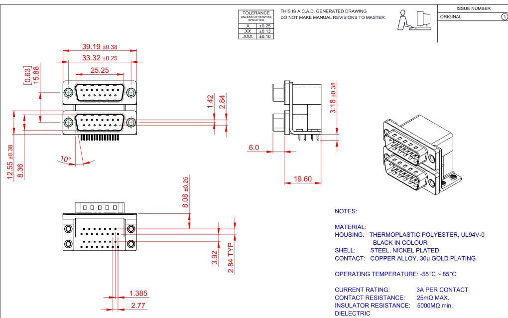
WITHSTANDING VOLTAGE: 1000V AC rms
