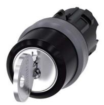
RONIS key-operated switch, 22 mm, round, plastic with metal front ring, lock number SB30, with 2 keys, 3 switch positions I-O-II, latching, actuating angle 2x45°, 10:30h/12h/13:30h, Key removal II, possible special locks: SB31, 421, 455 Z=50-unit packaging
