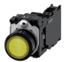
Illuminated pushbutton, 22 mm, round, plastic, yellow, pushbutton, flat, momentary contact type, with holder, 1 NO+1 NC, LED module with integrated LED 110 V AC, spring-type terminal, with laser labeling, lower case
