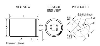
General Information Series ALC80 Dielectric Aluminum Electrolytic Description Snap-In, Aluminum Electrolytic RoHS Lead 3 Pin Short AEC-Q200 No Halogen Free Yes Component Weight 125 g Notes Dimensions D And L Include Sleeving. Shelf Life 156 Weeks
