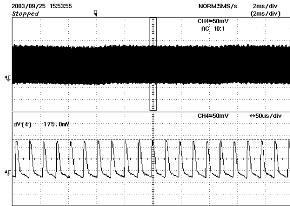
Figure 24 - Ripple, 230 VAC, Full Load. 2 ms, 50 mV / div.
