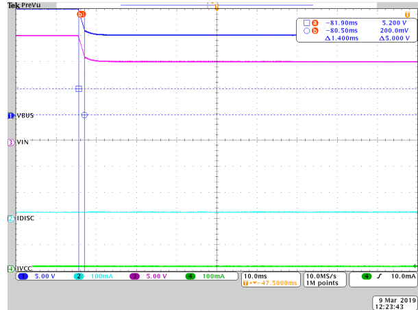
Figure 46. VBUS Discharge, from 20 V to 15 V, with a 2 A Load
