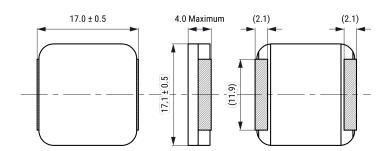
**General Information** Series MPX Style SMD Chip Size 1740(6868) Description Surface Mount Inductor Features Power Inductors **RoHS** Yes Core Composite Miscellaneous 40 (K) Temperature Rise Max.
