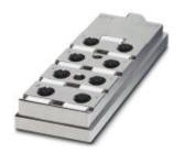
Sensor/actuator box, connection method: M12 socket Metal, number of slots: 6, number of positions: 5, coding: A - standard, slot assignment: Parallel, status display: No, Universal, shielding: yes
