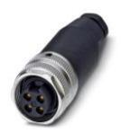
Connector, Universal, 4-position, Socket straight 7/8"-UNF, A-coded, Screw connection, knurl material: Zinc die-cast, nickel-plated, cable gland Pg9, external cable diameter 6 mm ... 8 mm
