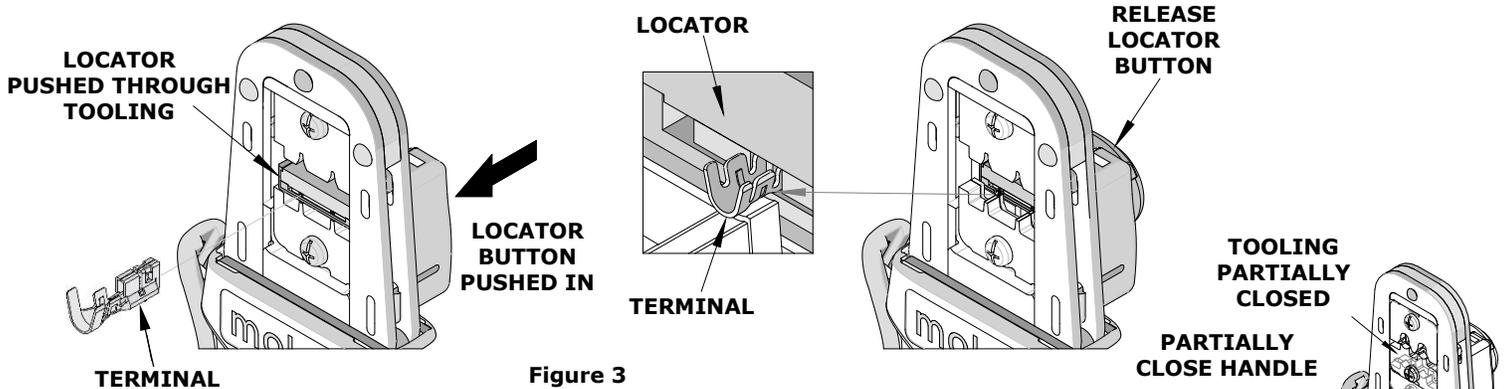
4. Release the locator button, allowing the locator to return to the crimping position.
