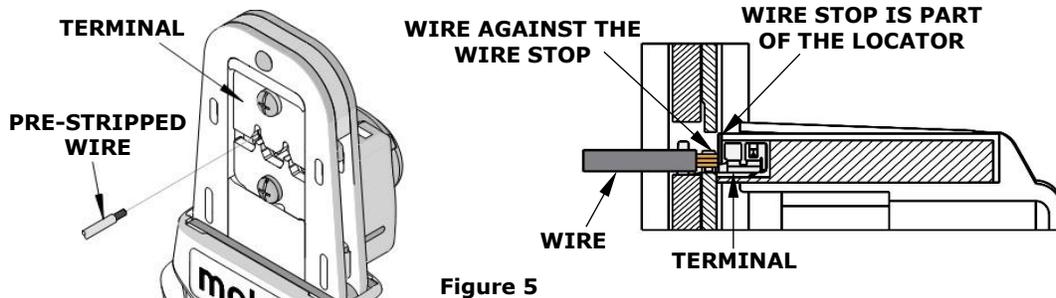
7. Crimp the terminal by squeezing the tool handles until the ratchet mechanism cycle has been completed. Release the handles to open the jaws.
