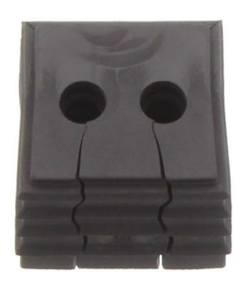
Seal, Mounting type: Plug in, Length x width: 20.3 mm, Max. cable diameter: 5 mm, IP 66, Colour: Black
