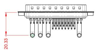
POWER/CO-AX CONTACT RATING:40A (CURRENT)(IF PRESENT)SIGNAL CONTACT CURRENT RATING:5A PER CONTACTSIGNAL CONTACT RESISTANCE: $10m\Omega$  MAX.INSULATOR RESISTANCE:5000MΩ min.DIELECTRICDIELECTRIC
