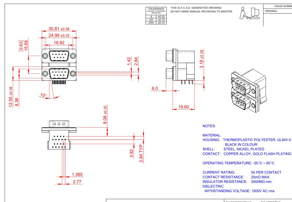
SW REFERENCE NO.: 661 ASSEMBLY 661 SERIES D-SUB CONNECTOR DRAWN: DATE: AUG. 01/2018 CHECKED: THESE DRAWINGS AND SPECIFICATIONS OF SCALE: 1:1 SHEET EDAC INC ARE THE PROPERTY OF EDAC INC..AND
