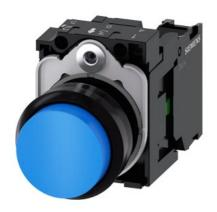
Pushbutton, 22 mm, round, plastic, blue, pushbutton, raised, momentary contact type, with holder 1 NO, screw terminal, with laser labeling, lower case
