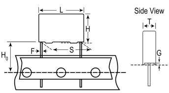
Style Radial Features MKP EMI Safety RoHS Lead Wire Leads Safety Class X1 Qualifications ENEC, UL, cUL, CQC AEC-Q200 No THB Performance No Component Weight 1.2 g Miscellaneous ClimCat: 40/110/56/C. Shelf Life 104 Weeks
