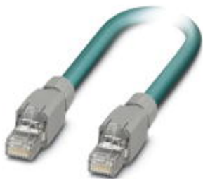
Assembled Ethernet cable, shielded, 4-pair, AWG 26 flexible cable conduit capable (19-wire), RAL 5021 (sea blue), RJ45 connector/IP20 to RJ45 connector/IP20, line, length 2 m
