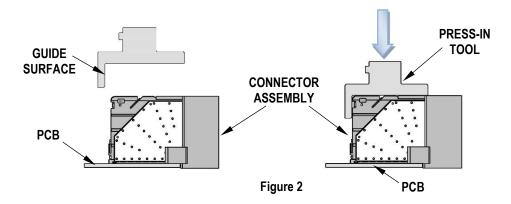
3. Using the application tool and an appropriate press, seat the Orthogonal Direct RAM module until there is less than 0.10mm (.004 in) clearance between the bottom of the plastic housing and the surface of the PCB. See Figure 3.
