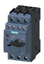
Special type Circuit breaker size S00 for motor protection, CLASS 10 A-release 4.5...6.3 A N-release 82 A screw terminal Standard switching capacity with transverse auxiliary switches 1 NO+1 NC Ambient temperature -50 °C 500 switching cycles
