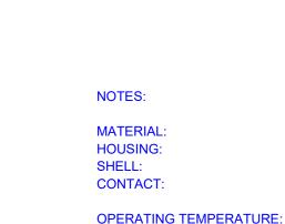
THERMOPLASTIC POLYESTER, UL94V-0 STEEL, NICKEL PLATED COPPER ALLOY, 30µ" GOLD PLATED
