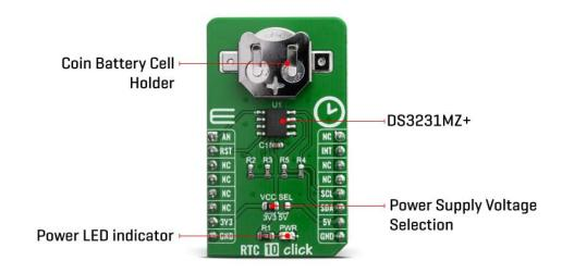
In addition to the DS3231M, RTC 10 click is equipped with the button cell battery holder compatible with the 3000TR batteryholder, suitable for 12mm Coin Cell batteries. By utilizing an automatic backup switch, the IC is able to use an external battery power source when there is no power supply on its main power terminals, thus allowing for uninterrupted operation.
