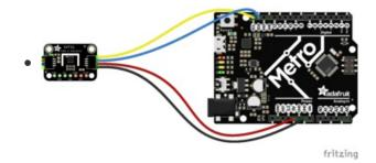
The SHT31-D has a default I2C address of **0x44** which you can change to **0x45** by connecting the **ADR** pin to the **VIN** pin
