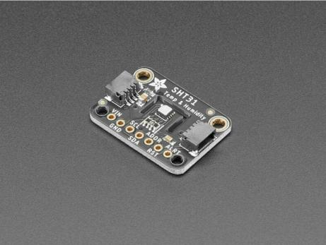
Sensirion Temperature/Humidity sensors are some of the finest & highest-accuracy devices you can get. And, *finally* we have some that have a true I2C interface for easy reading. The **SHT31-D** sensor has an excellent  $\pm 2\%$  relative humidity and  $\pm 0.3$ °C accuracy for most uses.
