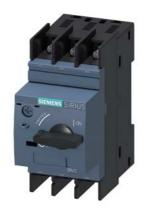
Circuit breaker size S0 for motor protection, CLASS 10 A-release 13...20 A N-release 260 A ring cable lug connection Standard switching capacity
