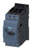
Circuit breaker size S2 for transformer protection A-release 18...25 A N-release 500 A screw terminal Standard switching capacity
