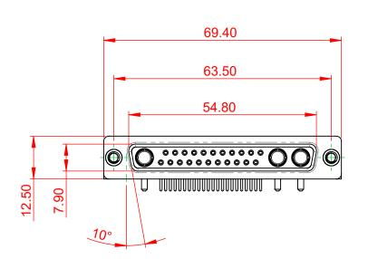
THIS IS A C.A.D. GENERATED DRAWING TOLERANCE UNLESS OTHERWISE SPECIFIED DO NOT MAKE MANUAL REVISIONS TO MASTER. .X ±0.25 .XX ±0.13
