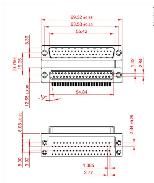
THIS IS A C.A.D. GENERATED DRAWING TOLERANCE UNLESS OTHERWISE SPECIFIED DO NOT MAKE MANUAL REVISIONS TO MASTER. .X ±0.25 ±0.13
