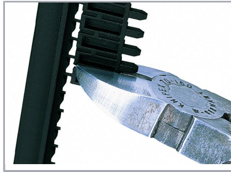
Remove unrequired sections from the sidewalls.
