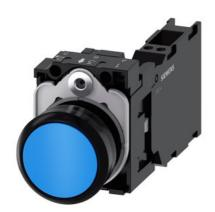
Pushbutton, 22 mm, round, plastic, blue, pushbutton, flat, momentary contact type, with holder 1 NO+1 NC, spring-type terminal, with laser labeling, inscription or symbol Customer-specific selection with SIRIUS ACT configurator (CIN)
