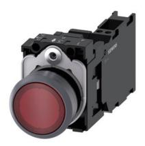
Illuminated pushbutton, 22 mm, round, plastic with metal front ring, red, pushbutton, flat, momentary contact type, with holder, 1 NO+1 NC, LED module with integrated LED 24 V AC/DC, spring-type terminal, with laser labeling, symbol number according to, ISO 7000 or IEC 60417
