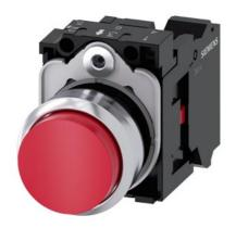
Pushbutton, 22 mm, round, metal, shiny, red, pushbutton, raised, momentary contact type, with holder, 1 NC, spring-type terminal, with laser labeling, lower case
