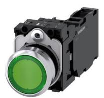
Illuminated pushbutton, 22 mm, round, metal, shiny, green, pushbutton, flat, momentary contact type, with holder, 1 NO+1 NC, LED module with integrated LED 24 V AC/DC, screw terminal, with laser labeling, upper case and lower case, Always upper case at the beginning of the word
