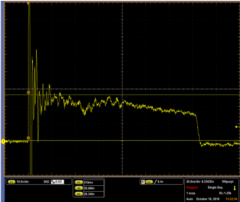
AQHV12-C +8kV Contact ESD Clamping Voltage
