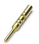
Crimp contact, turned, contact diameter: 0.8 mm, crimp range: 0.34 mm<sup>2</sup> ... 0.5 mm<sup>2</sup>
