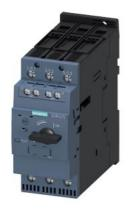
Circuit breaker size S2 for motor protection, CLASS 10 A-release 18...25 A N-release 325 A screw terminal increased switching capacity with transverse auxiliary switches 1 NO+1 NC
