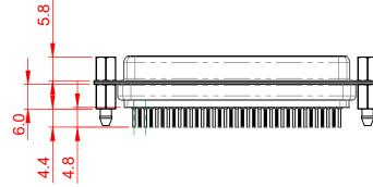
CONTACT RESISTANCE: 25mQ MAX. INSULATOR RESISTANCE: 5000MΩ min. DIELECTRIC WITHSTANDING VOLTAGE: 1000V AC rms
