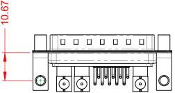
75Ω (IMPEDANCE) POWER/CO-AX CONTACT RATING: (IF PRESENT) SIGNAL CONTACT CURRENT RATING: 5A PER CONTACT SIGNAL CONTACT RESISTANCE:  $10m\Omega$  MAX. **INSULATOR RESISTANCE:**
