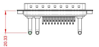
30A (CURRENT) **POWER/CO-AX CONTACT RATING:** (IF PRESENT) SIGNAL CONTACT CURRENT RATING: 5A PER CONTACT SIGNAL CONTACT RESISTANCE:  $10m\Omega$  MAX. **INSULATOR RESISTANCE:** 5000MΩ min. DIELECTRIC
