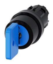
Key-operated switch O.M.R, 22 mm, round, plastic, lock number 73038, blue, with 2 keys, 3 switch positions I-O-II, latching, actuating angle 2x45°, 10:30h/12h/13:30h, Key removal I+O+II, with laser labeling, inscription or symbol Customer-specific selection with SIRIUS ACT configurator (CIN)
