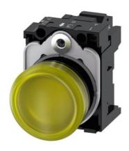
Indicator lights, 22 mm, round, plastic, yellow, lens, smooth, with holder, LED module with integrated LED 110 V AC, spring-type terminal, Z=20-unit packaging
