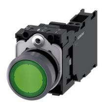
Illuminated pushbutton, 22 mm, round, plastic with metal front ring, green, pushbutton, flat, momentary contact type, with holder, 1 NO+1 NC, LED module with integrated LED 24 V AC/DC, spring-type terminal, with laser labeling, lower case
