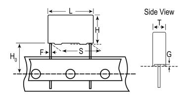
Series F461 Dielectric Metallized Polypropylene Style Radial MKP, Pulse Features RoHS Yes Lead Wire Leads AEC-Q200 No Component 0.625 g Weight The Rated Voltage Decreases 2%/C Between +85C And +105C (1.25%/C For AC). ClimCat: Miscellaneous 55/105/56. Notes Series Replaced by R75.
