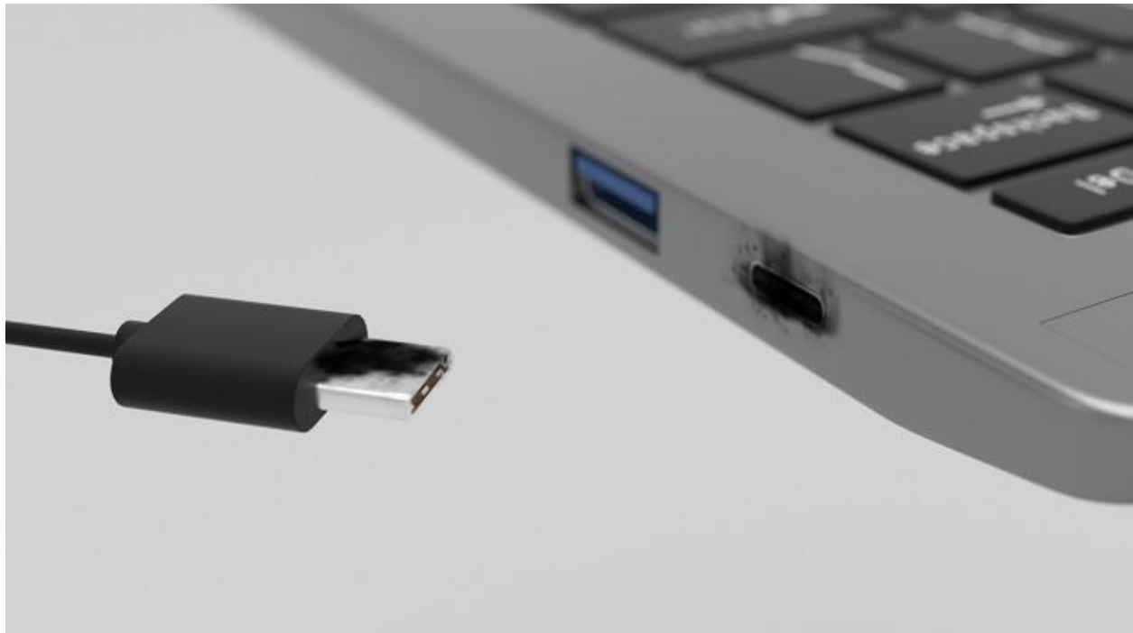
Fig. 1: Resistive faults in USB-C connectors can damage both cables and the devices being charged.
