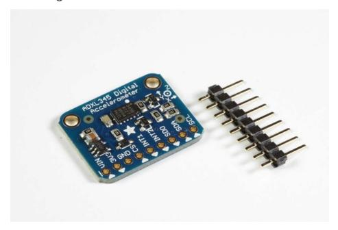
The board comes with all surface-mount components pre-soldered. The included header strip can be soldered on for convenient use on a breadboard or with 0.1" connectors. However, for applications subject to extreme accelerations, shock or vibration, locking connectors or direct soldering is advised.
