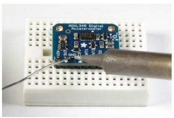
And Solder! Be sure to solder all pins to assure good electrical contact.
