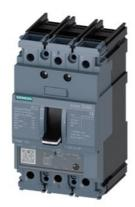
circuit breaker 3VA5 UL frame 125 breaking capacity class M 35kA @ 480 V 3-pole, line protection TM230, FTAM, In=20A overload protection Ir=20A fixed short-circuit protection Ii=7.5...15 x In nut keeper kit on both sides
