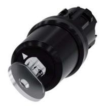
key-operated switch Siemens, 22 mm, round, plastic, lock number SSG10, with 2 keys, 2 switch positions O<I, momentary contact type, actuating angle 45°, 10:30h/12h, key removal O, with laser labeling, inscription or symbol customer-specific selection with SIRIUS ACT configurator (CIN)
