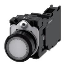
Illuminated pushbutton, 22 mm, round, plastic, clear, pushbutton, flat, momentary contact type, with holder, 1 NO+1 NC, LED module with integrated LED 110 V AC, spring-type terminal, with laser labeling, inscription or symbol Customer-specific selection with SIRIUS ACT configurator (CIN)
