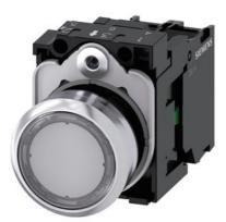
Illuminated pushbutton, 22 mm, round, metal, shiny, clear, pushbutton, flat, momentary contact type, with holder, 1NO, LED module with integrated LED 24 V AC/DC, screw terminal, with laser labeling, inscription or symbol Customer-specific selection with SIRIUS ACT configurator (CIN)
